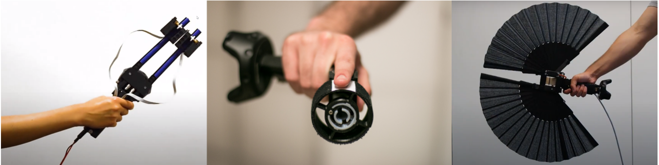
Figure 1: a selection of hand held haptic feedback devices, on the left the Transcalibur [12] a device for 2d shape rendering, in the middle is the Haptic Revolver [21] which is able to render surfaces and on the right is the Drag:on [24] which is able to simulate different aspects of a virtual object using drag force
