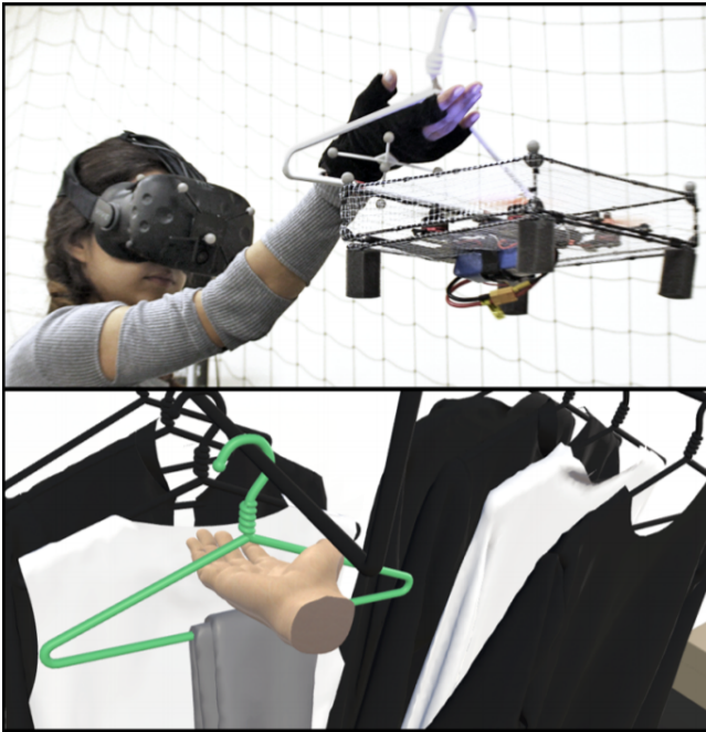
Figure 9: Interaction with a passive object attached to the HoverHaptics drone [2]
