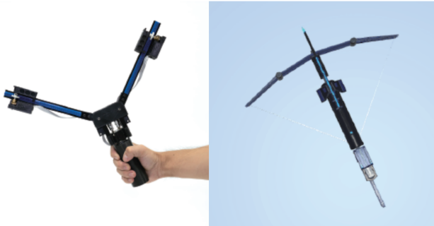
Figure 5: The Transcalibur device [12] rendering a shape
